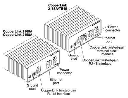
Figure 2. CopperLink Ethernet Extender rear panel
